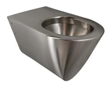
Conical wall hung toilet extended version for P.R.M with wall fixations in stainless steel quality AISI 304 18/10 (1.4301), 1,5 mm thickness, brushed finish. One-piece stamped toilet bowl, anti-splash shape. European Standard EN-997:2012 Class 1 Type 4A, 4C minimum flush 4 or 6 L and CE.
