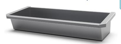
Collective wash through made in stainless steel quality AISI 441, satin finish. Side thickness 1,5 mm / basin 0.8 mm.
