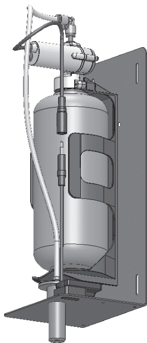
1 X PUMP, MOUNTING PLATE, BOTTLE SUPPORT, AND SOAP TANK WITH SPOUT AND SENSOR
