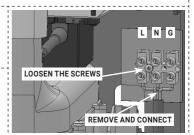
Instead, screw on the bare-wire power supply cable connected to the electrical terminal.
