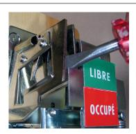
In case of obstruction, use leverage to remove the unwanted object.
