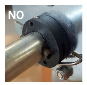
2. Return the key to the FREE position: turn it until the FREE indication appears (rotate right for locks n°1 and 3, or rotate left for locks n°2 and 4).
