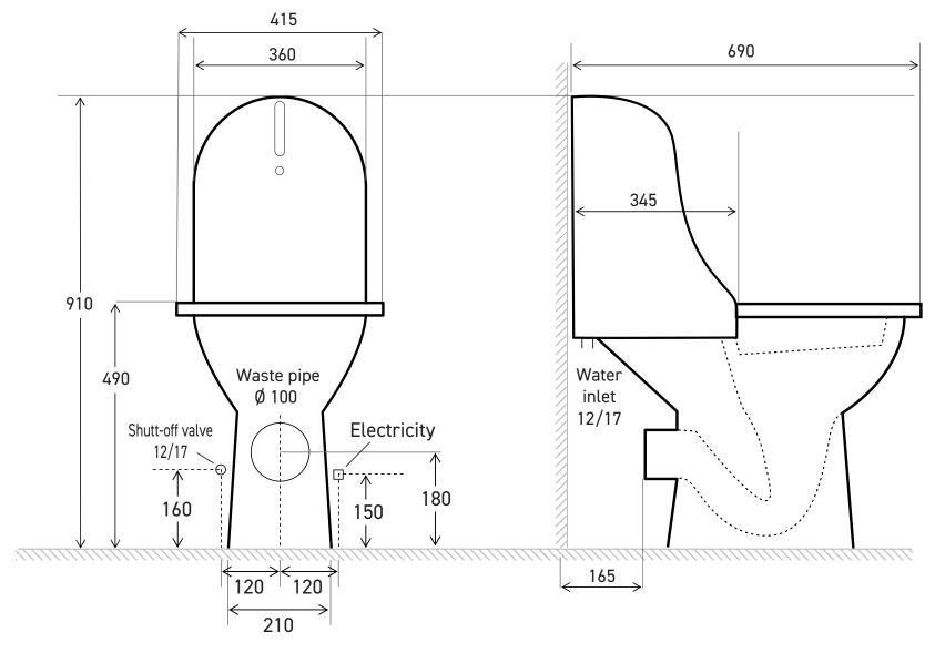
Power supply via 12V/220V transformer concealed behind the unit. If possible, install in a location protected from splashes and theft (utility room, adjacent room, false ceiling, etc.).
