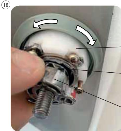
To turn "the nut to the 3 equidistant branches" - located between the POM ring in the integrated spring and the nut to the 3 red O rings -
