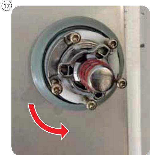
**To unscrew** by a few turns "the nut with the 3 red O rings", **while turning it anti-clockwise**.
