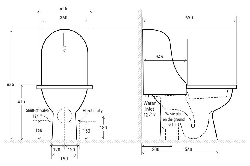
Power supply via 12V/220V transformer concealed behind the unit. If possible, install in a location protected from splashes and theft (utility room, adjacent room, false ceiling, etc.).
