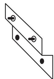
**ÉTAPE 2****Fixation au mur du rail de suspension du module**
